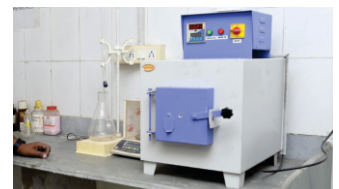
Muffle Furnace Test
